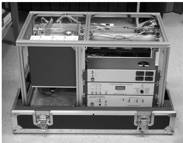
Figure 5 The PI/QitToF without panels or autosampler configured for "fly-away" applications. Computer and roughing pump not shown.
